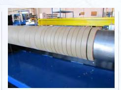
The TAM-01S is a manually operated machine, which is designed for low volume core users who cannot justify a high capital outlay. Operation and set up is simple utilising two hand operation for complete safety.
